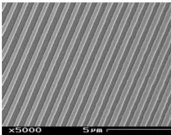
Figure 4. A template directing the uniform assembly of block copolymers.
